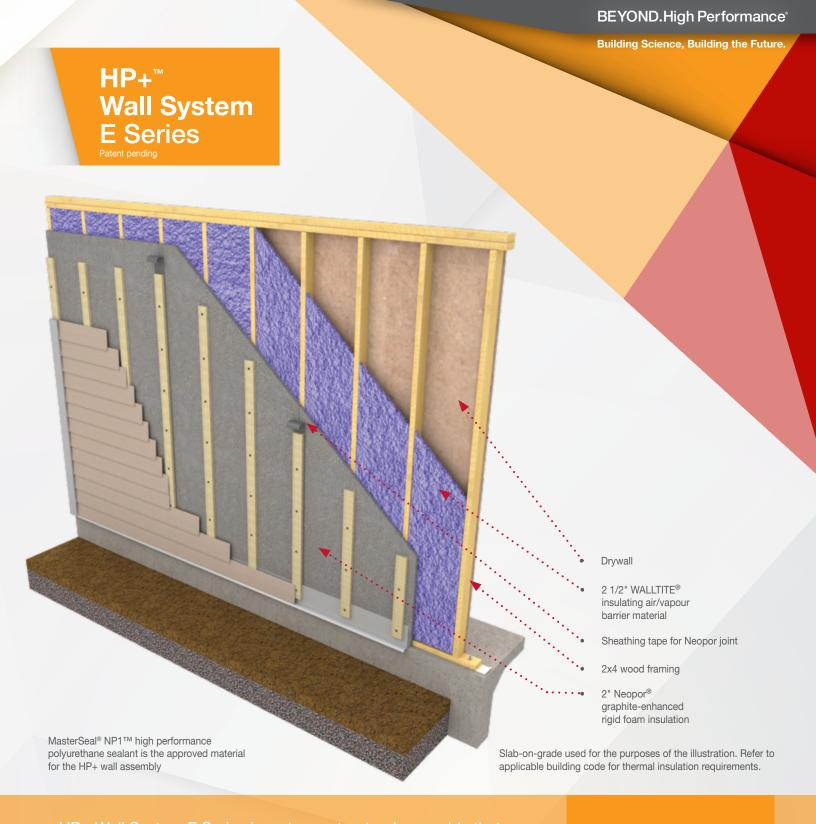
HP+ Wall System E Series is a strong structural assembly that meets or exceeds codes with a minimum nominal insulation R-value of R-25 up to R-32 with 2x4 wood framing. The E Series offers exceptional energy and cost efficiencies.
